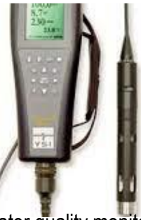
YSI (water quality monitoring unit)
